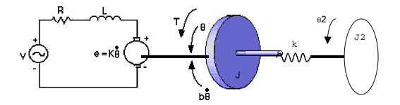
Fig. 1 Schematic diagram of DC motor with Load
